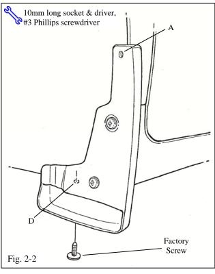
(c) Hold the part up and into the body panel and reinstall the OE screw into location D (Fig. 2-2).
